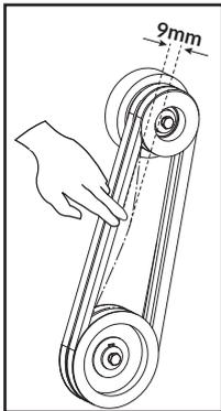
The belt has to have a tension such that when pressed with the fingers it can flex 9mm. To adjust the belt tension, the motor must be displaced, to do this:
